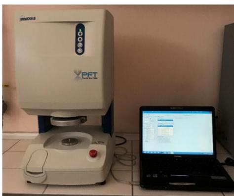
Figure 2. Powder flow tester
