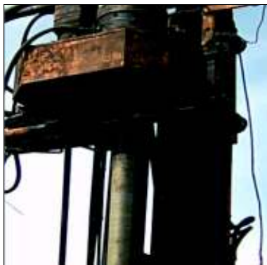
Picture 7: Detail of the string and clamp rotation
