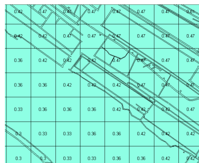
Figure 1. Unit Risk Probability of the V_{9-10} Coal Seam of the Eighth Mine of Pingdingshan
