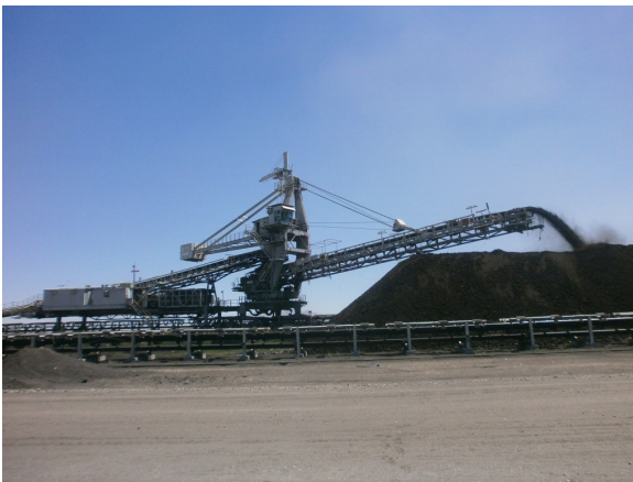
Photograph 2. Windrow stacking at Afşin-Elbistan Stockyard
