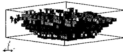
Figure 3. Three-dimensional ore body block model.
