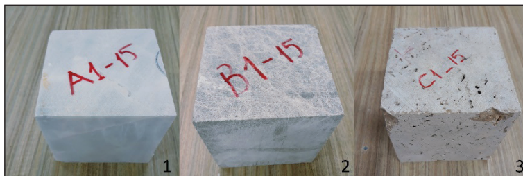
Figure 1. Pre-thermal damage (original samples)
