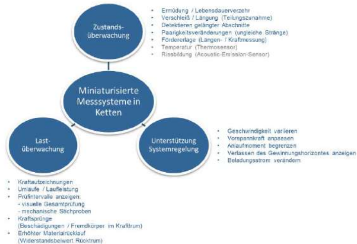
Figure 10: Schematic diagram of a comprehensive chain monitoring system
