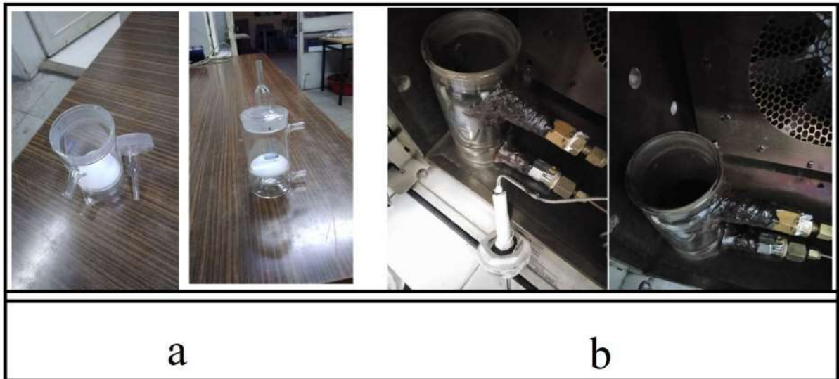
Figure 4. Quartz modified reactor for the experimental set up (new) of spontaneous combustion tests (a: before modification, b: after modification).
