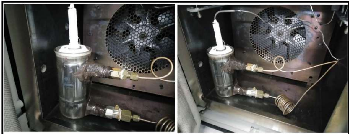
Figure 5. Copper pipes connected to the reactor.
