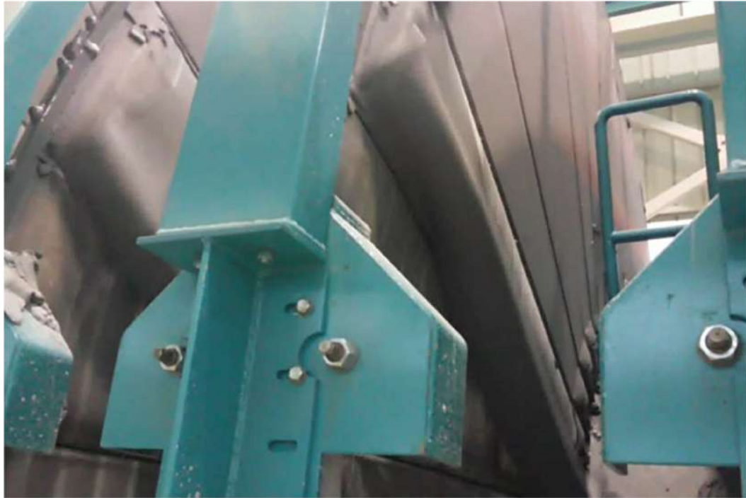
Figure 5. Tailings dewatering from a gold/silver mine with a Boozer disc filter L4 (176 m 2 filter area) – complete cake discharge during pre-commissioning
