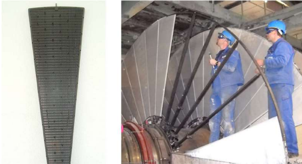
Figure 2. New lightweight snap-on segment of only 12 kg in weight (left), mounting of new segments (right)
