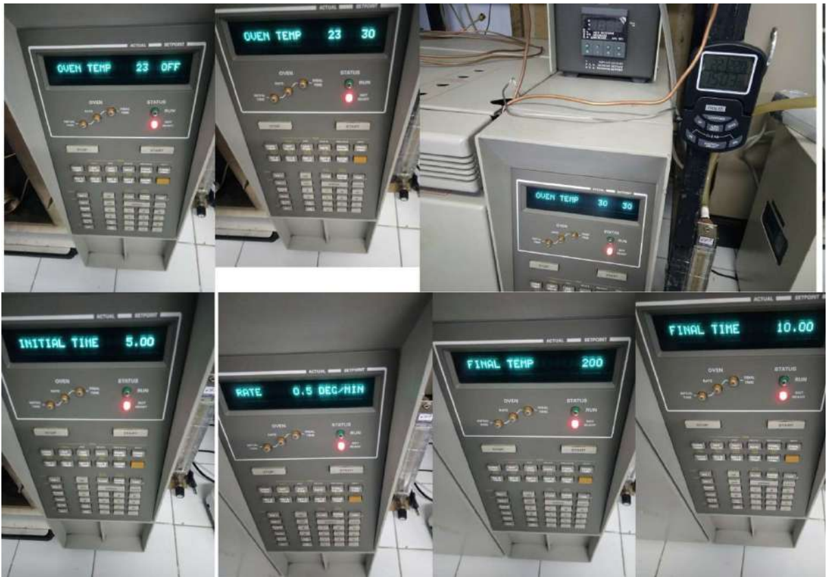
Figure 3. Temperature programming of the oven in the body of GC.
