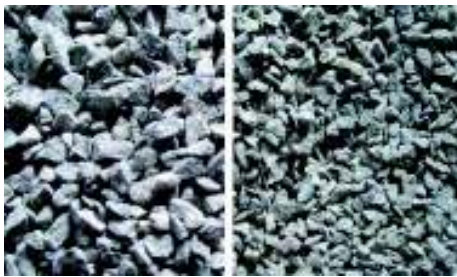
Figure 3. At the right, material retained on 25.4 mm; at left, material between 6.3 mm and 4.7 mm
