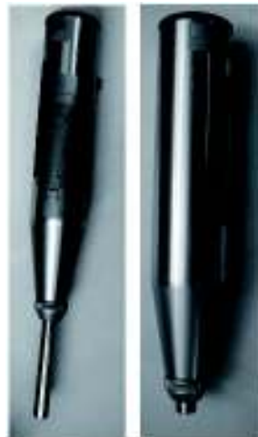
Figure 2. Schmidt hammer (N type - 2.207 Nm impact energy) with retractable impact plunger at starting and ending position (locked by pressing the pushbutton after impact, allowing scale reading).
