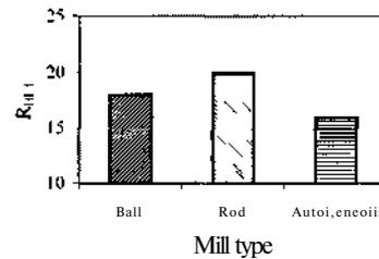
Figure 5 The BET surface roughness (R<sub>BET</sub>) values of calcite mineral ground in different mills
