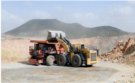
Photograph 1. L-1350 is loading to Hitachi EH400AC-3 truck at the gold mine
