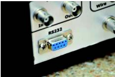
Picture 3. The RS232 DB9 connector for PC communication and/or direct printing
