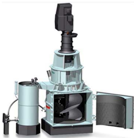
Figure 1. Illustration of a Metso brand Vertimill (Metso, 2017)
