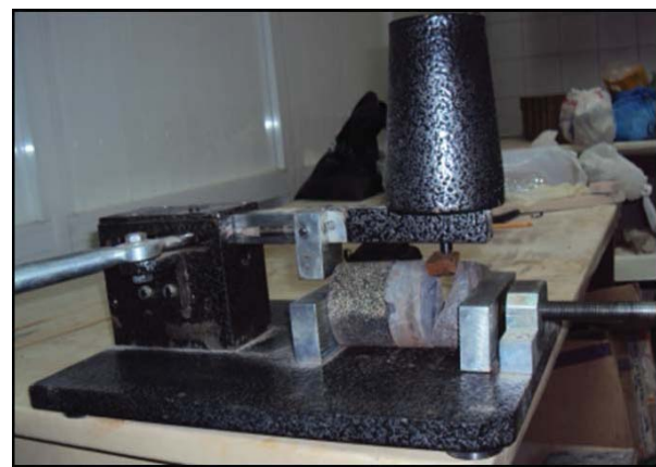
Figure 3. Cerchar test apparatus.
