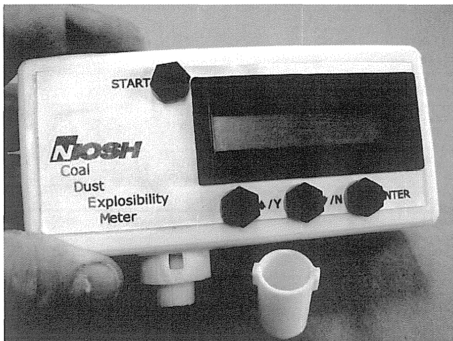
Figure 4. Coal Dust Explosibility Meter (CDEM).
